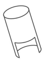
Tube 1: (Top) Cut the upper jaw out of the tube, approx 1/3 of the way up it.
